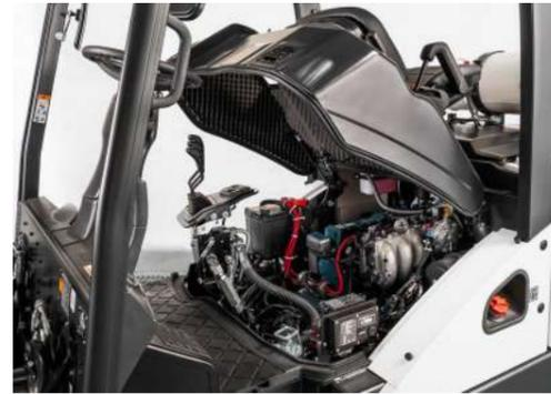
Easy access to main components with a tool-less removable floor plate and a hood that opens 60 degrees
