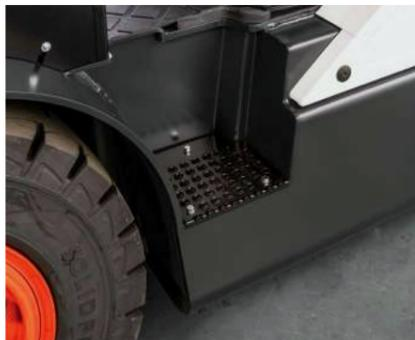
This forklift features a low step height, facilitating easy and safe operator entry and exit, complemented by an entry grab bar and an anti-slip step plate.
