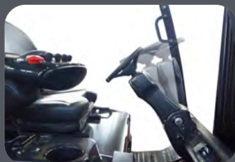
Fully Adjustable Steering Column
